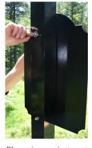
Place sign against post inserting studs through holes. Fasten sign to post with provided washers and acorn nuts using a 7/16" wrench.
